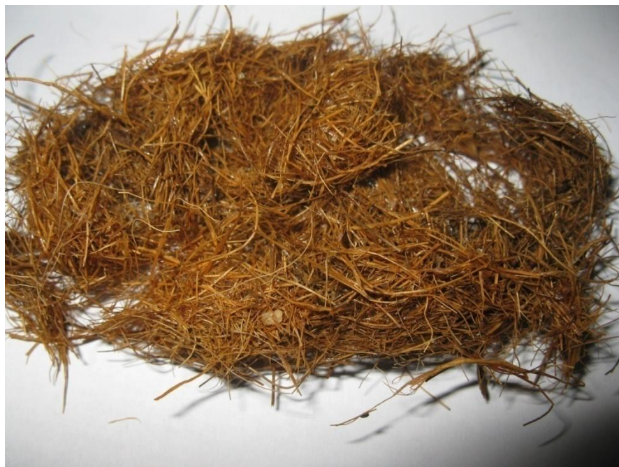
Non woven coir geotextiles taken from Kozhinada road after 4 years
