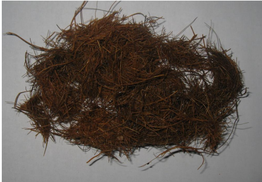
Non woven coir geotextiles taken from Kozhinada road after 4 years
